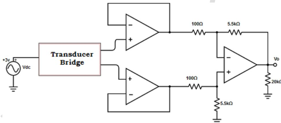
Consider the entire resistors in the bridge circuit are equal. The resistance and change in resistance are given as  $3k\Omega$  and  $30k\Omega$ . Calculate the output voltage of differential instrumentation amplifier?
