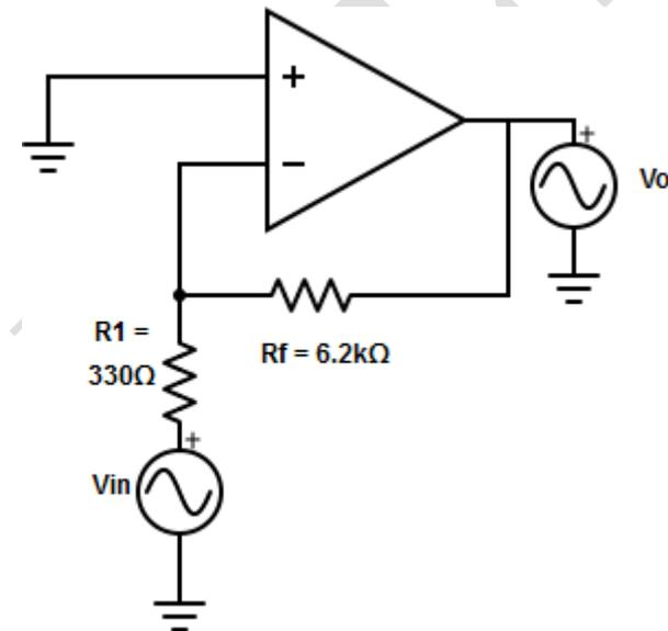
Compute the value of output resistance, bandwidth and closed loop voltage gain for the circuit shown.
