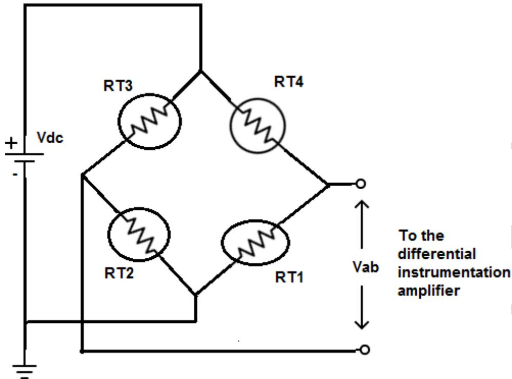
$R_{T1}$ ,  $R_{T2}$ ,  $R_{T3}$ ,  $R_{T4}$  are unstrained gage resistance. If the resistance change in each gage is  $0.3\Omega$ . Choose the correct option?
